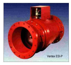
from an explosion detector causing a gas generator to assist the valve in closing. It is used where the force of an explosion is not expected to generate enough pressure to shut the valve without assistance. The Ventex ESI-P's fast isolation speed and enhanced design make it extremely well suited for St3 class dusts of up to a KST of 500 bar-m/sec and pressures of up to 300 psi ( 20 bar ).
