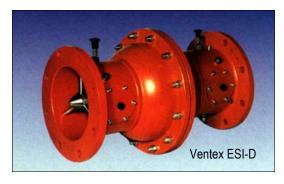
**The Ventex ESI-D** is a passive acting dual direction valve which is closed by the pressure wave of the explosion. They are used in places where the explosion can occur in either direction. Valves are available in sizes from 4 to 20 inches nominal diameter.
