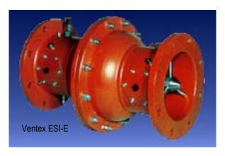
The **Ventex ESI-E** is a passive acting, single direction valve which is closed by the pressure wave of the explosion. They are applied in areas where the explosion can only come from one direction. Valves are available in sizes from 4 to 28 inches nominal diameter. The maximum airflow through the valve in the closing direction is 66 ft/sec.
