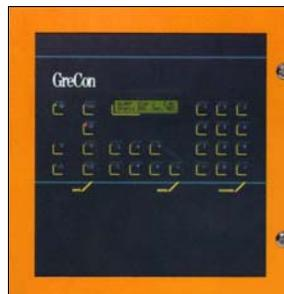
To protect conveyors or other areas subject to ambient light, GreCon has available a sensor that responds only to the movement of invisible infrared radiation. The GreCon Control Panel can handle up to 24 independent areas.
